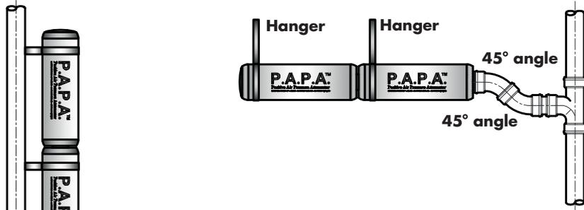
When mounting the P.A.P.A. devices vertically or horizontally each P.A.P.A. device should be independently supported by an anchor connected to its housing as shown. The anchor's metal hoop around the P.A.P.A. housing unit should allow for expansion and contraction and be rubber lined to prevent damage.
