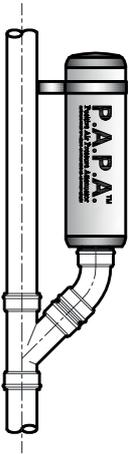
When mounting the P.A.P.A. device vertically the P.A.P.A. device should be independently supported by an anchor connected to its housing as shown in the left diagram. The anchor's metal hoop around the P.A.P.A. housing unit should allow for expansion and contraction and be rubber lined to prevent damage. Alternately, the P.A.P.A. should be connected to the pipe with the use of a no-hub coupling or flexible coupling.
