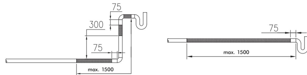
■ Mini-Vent should be installed in these areas
