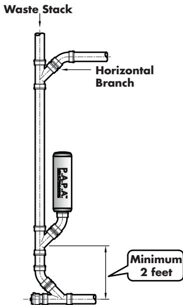
Stack extending no more than 5 floors above the base of the stack or offset should be a minimum of 2 feet
