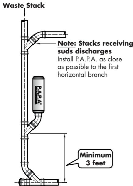
Stack extending no more than 5 floors above the base of the stack or offset should be a minimum of 3 feet
