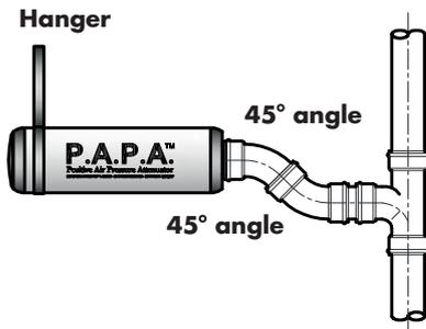
When mounting horizontally (it is advisable to maintain a minimum of a few degrees of slope so as to induce self draining), or at any angle up to 90 degrees, the P.A.P.A. device should be supported or anchored as shown in the left diagram. The portion of the support or anchor in contact with the device housing should allow for expansion and contraction and be rubber lined to prevent damage.
