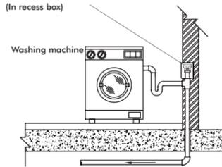
BRANCH VENT WITH FLOOR DRAIN
